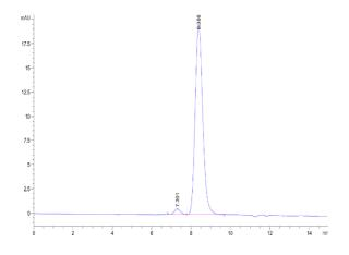
The purity of Biotinylated Human EGFR is greater than 95% as determined by SEC-HPLC.
