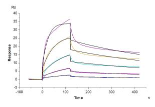
Biotinylated Human EGFR, His Tag captured on CM5 Chip via Anti-his antibody can bind Human EGF, No Tag with an affinity constant of 0.62 nM as determined in SPR assay (Biacore T200).
